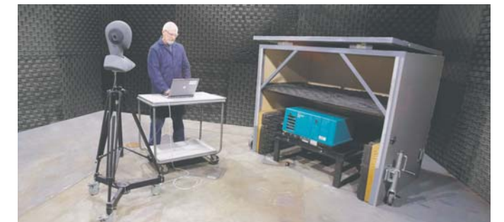
High-tech binaural recording system enables Cummins Onan to fine-tune generator noise characteristics.
